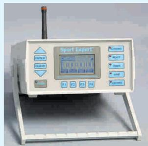
The MCU features 4 RISC type processors operating in parallel, which allows an excellent performance of the system. The system can store up to 1500 user (athlete) files in the memory of MCU.
